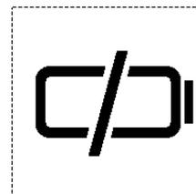
The battery is exhausted. Replace the batteries.
