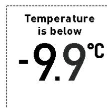
Frost can damage the sensor. The recommended operating temperature of the sensor is 0 °C to 50 °C (32 °F to 122 °F).
