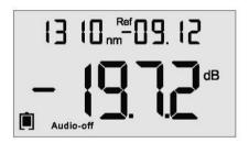
(7). If to measure the loss of optical fiber link, it is necessary to carry out local initialization reference for light source and optical power meter, as shown in the following Fig, read the initial reference value on optical fiber meter, and it is available to press the key continuously to save this reference value.
