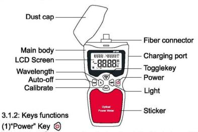
Shout press to turn on the device, the default is to turn off the device after 1 hour.
