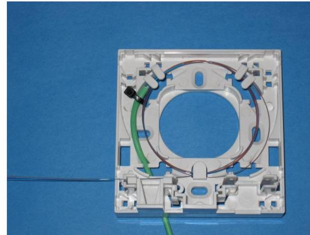
Placing 1st pigtail and splice
