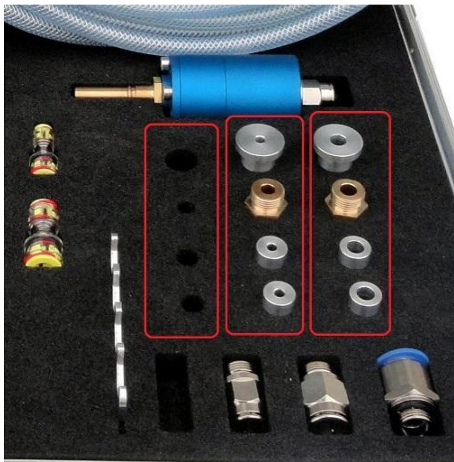
Fig. 15 Sleeves arranged in groups depending on the diameter of the cable
