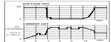
The output of the device is electrically protected against overload and short circuit. For the nominal voltage and nominal current at temperature condition, please see technical data. The device can supply at the nominal Current without switching off. As the overload increases, the output voltage is reduced until zero.
