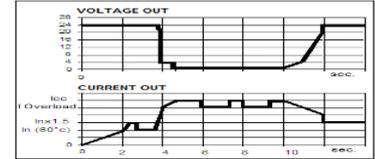
The output of the device is electrically protected against overload and short circuit. For the nominal voltage and nominal current at temperature condition, please see technical data. The device can supply at the nominal Current without switching off. As the overload increases, the output voltage is reduced until zero.
