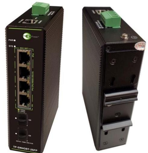
The switches require a 48VDC to 57VDC input on the dual input wire terminal connector which is capable of accepting up to 12AWG wire.
