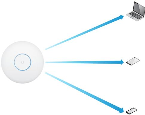
MU-MIMO with 2x2 and 1x1 clients: The UniFi AC HD AP communicates with one 2x2 client and two 1x1 clients at a time.
