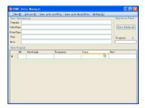
Connect the Optical Multimeter FHM2 and computer with the USB cable, and turn the instrument on. Click the "Data download" Botton to download the test results.
