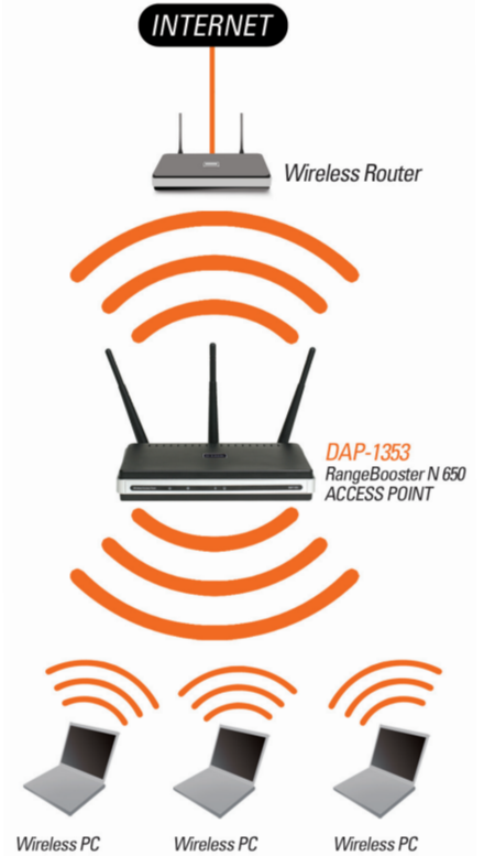
Extending the wireless coverage of a wireless router using the DAP-1353
